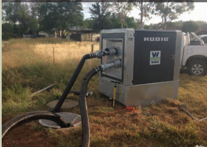
The Hüdig Electric-Vacuum-Unit has an electric driven water and vacuum-pump
